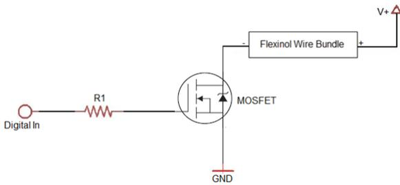
Figure 4. MOSFET switching circuit
