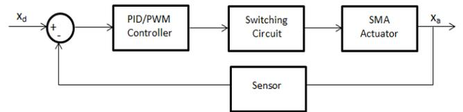
Figure 2. Actuator control system.
