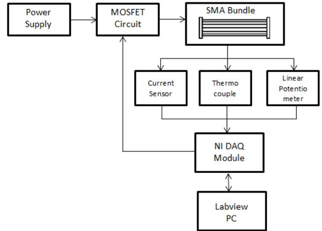
Figure 5. Actuator system block diagram
