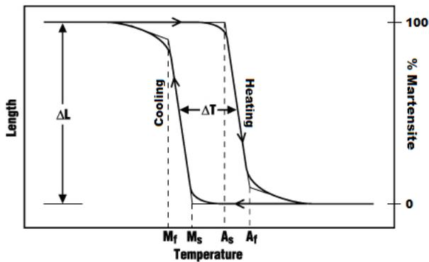
Figure 1. SMA thermo-mechanical hysteresis [1]
