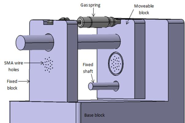
Figure 3. Actuator structure final design.
